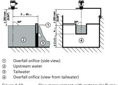
Figure 4.10 Flow measurement with rectangular flume: h<sub>max.</sub> = max. filling of the rectangular flume
