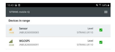
Click on the device you wish to connect to. On first connection, a PIN code shipped with the device needs to be entered (see *Device Bluetooth and Parameter Access Codes* sheet). Following successful PIN entry, the device cockpit will be shown.
