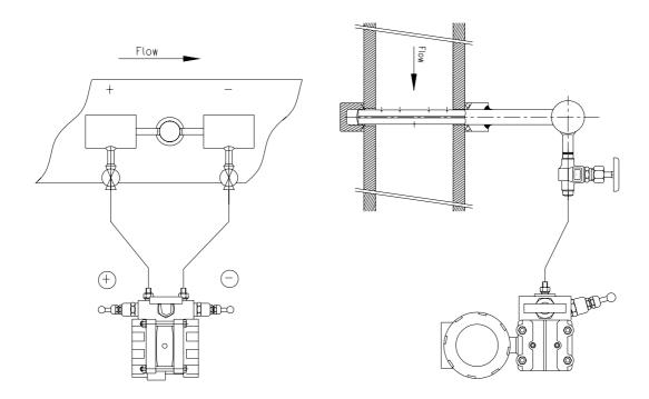
figure 2: Steam flow measurement in a horizontal and a vertical pipe
