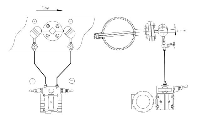
figure 1: Steam flow measurement in a horizontal pipe with a slope of 5 degr.
