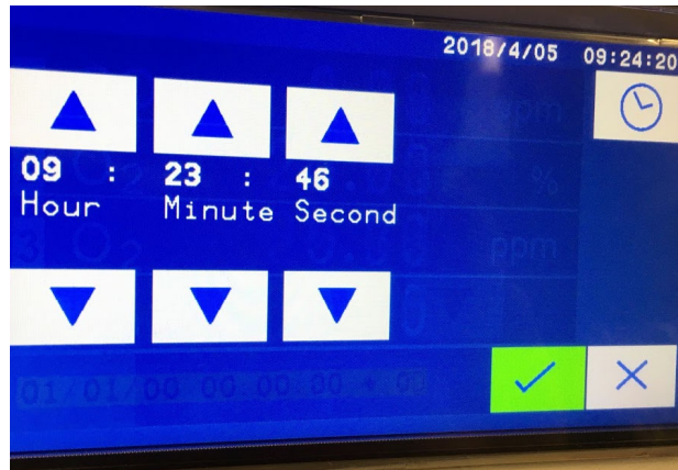
Figure 11-18: Set the analyzer Time Screen
