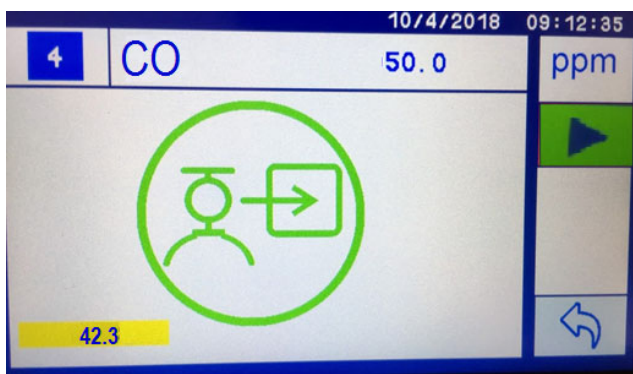
Figure 12-4: Start calibration – READY State
