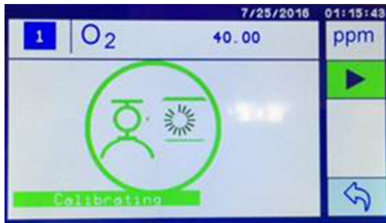
Figure 12-7: Calibration or Validation “Service In Progress” screen
