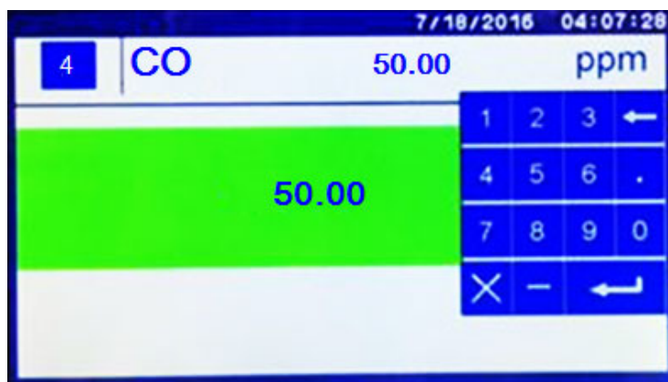
Figure 12-2: Span value entry keypad with Target Value on the top bar
