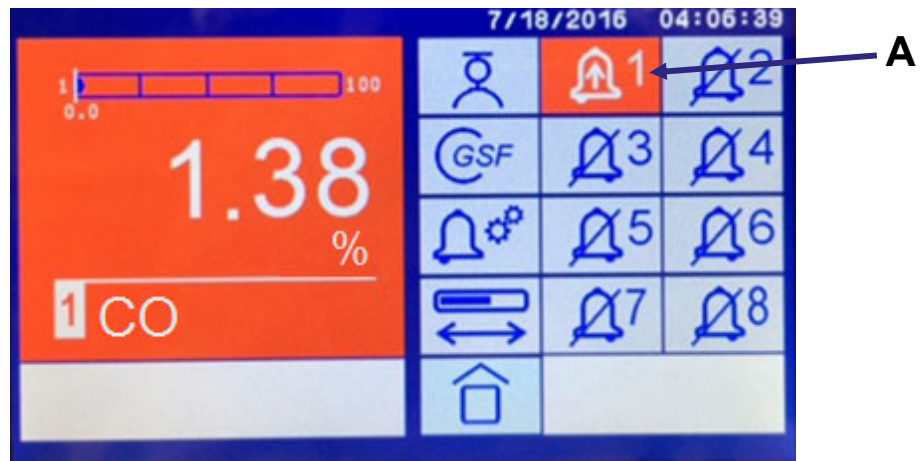
Figure 8-13: Alarms screen showing Alarm #1 (A) High Measurement Range triggered
