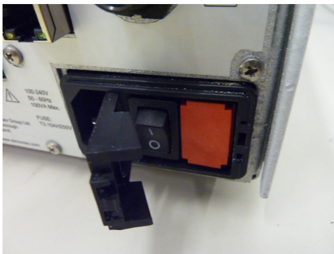
Figure 14-2: Fuse panel opened
