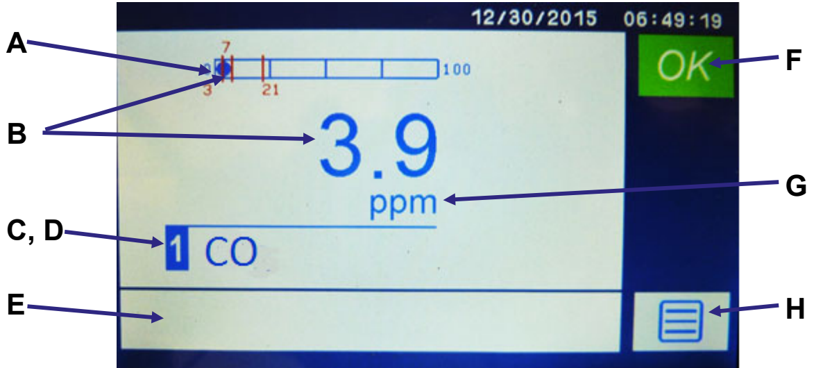
Figure 6-4: Single Gas Home screen components
