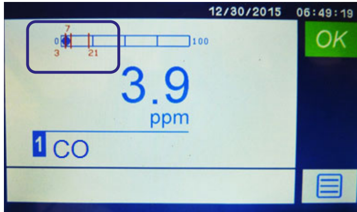
Figure 8-10: Home screen showing alarm settings as red lines and text on the bar graph
