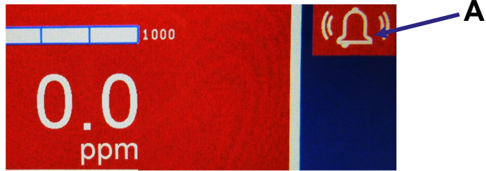
Figure 8-12: Measurement alarm condition triggered
