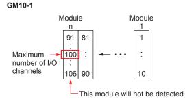
• If you want to use the DI of a GX90XD or GX90WD, only a single module installed in the GM main unit can be used.
